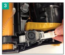
Pull up white latch to release the belt assembly and lift straight out.
